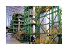
Pickled hot rolled coils are zinc-coated directly (GHR) or after cold rolling (GCR) by continuous hot-dip method on the galvanizing line. Galvanized coating process is applied to both lower and upper surfaces.
