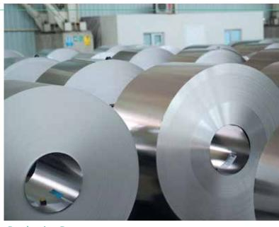
Tinplate products are produced by electrolytic chromium or tin coating of cold-rolled low carbon flat steel. Both surfaces can be coated in equal or different weights of tin coating.
