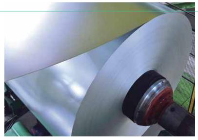
These products are produced by hot-dip galvanizing of both surfaces of the cold-rolled flat steels or pickled hot-rolled flat steels.
