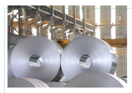
The Pickled and Hot Rolled Products are produced by cleaning the scale layer of hot rolled products with Hydrochloric Acid in the continuous pickling line. Pickled products are preferred in places where surface cleaning is important in terms of surface appearance.
